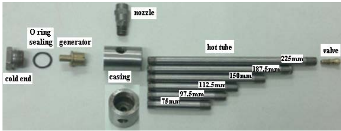
Fig. 2. Fabricated Vortex Tube with different tube length
